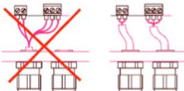
Please protect all of the power supply and control cables in front of the terminals mechanically by using suitable measures against unintentional loosening.
