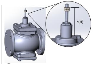
Position Jam nuts as per reference drawing and lock nuts together.
