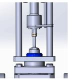
Thread the valve stem into the coupling until the jam nuts meet the coupling. Lock the upper jam nut against the coupling. Lock the second jam nut against the upper nut.
