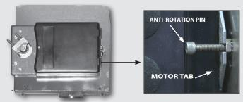
An anti-rotation pin engages a slotted tab at the foot of the motor to allow alignment of the motor as its shaft clamp rotates. The pin (screw) threads into a boss on the linkage base and is retained by a locking nut.
