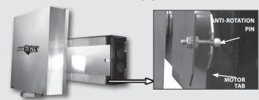
An anti-rotation pin engages a slotted tab at the foot of the motor to allow alignment of the motor as its shaft clamp rotates. The pin (screw) passes through the "Hi-Temp Motor Mounting Bracket, and is retained by "KEP" nuts on either side of the sheet metal.
